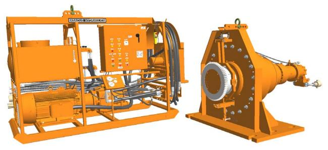
The drive units are equipped with the exclusive TORFLEX® gear type coupling which has been specifically designed and developed by Abacus Hydraulics Ltd. Small size couplings are equipped with manual shifter mechanism while all medium to large size couplings are standard equipped with hydraulically assisted shifter mechanism.
